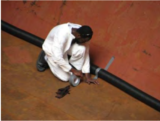
Plastic tubing is taped to the perimeter of the cargo hold.
