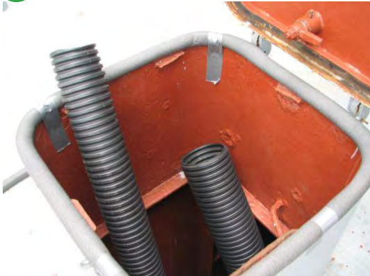
A blower is attached to the J-System® tubing inside the manway opening allowing high fumigant concentrations from the surface of the cargo to be forced to the bottom of the cargo hold.
